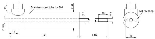
Version with ball joint on plunger (KV) (without rod guide)
