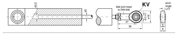
Version with ball joints on plunger (KFN) and on end of case (KFH) (with rod guide, captivated)
